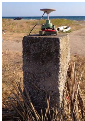
Figure 11: The LEICA SR520 receivers during the GPS measurements on BMs in Thessaloniki.
