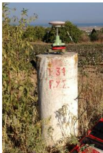
Figure 11: The LEICA SR520 receivers during the GPS measurements on BMs in Thessaloniki.
